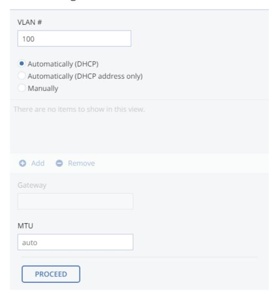
5. On the **Assign network** panel, select a network to connect the VLAN network interface to (for details, see *Managing Networks and Traffic Types* (page 2)) and click **Done**.
