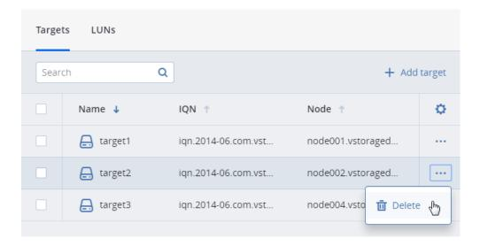
If you delete a target on the Active/Optimized path (indicated in LUN details), said path will switch to another target.
