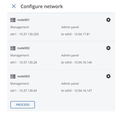
5. Next, on **Configure network**, provide one or more unique static IP addresses for the highly available admin panel, compute API endpoint, and interservice messaging. Click **DONE**.
