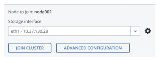
4. Click **Join cluster** to have Acronis Software-Defined Infrastructure assign the roles to disks automatically and add the node to the current cluster. Alternatively, click **Advanced configuration** to assign the roles to each drive manually (see *Assigning Disk Roles Manually* (page 15)).
