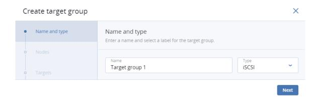
2. On **Nodes**, select nodes to add to the target group. On these nodes, iSCSI targets will run. You can only choose nodes with network interfaces that are assigned the **iSCSI** traffic type. It is recommended to have at least two nodes in the target group to achieve high availability. If you plan to use multiple iSCSI initiators, you should have as many nodes in the target group.
