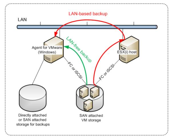
eliminate transferring the backed-up data via LAN, store the backups on a local disk of the agent's machine or on a SAN attached storage.
