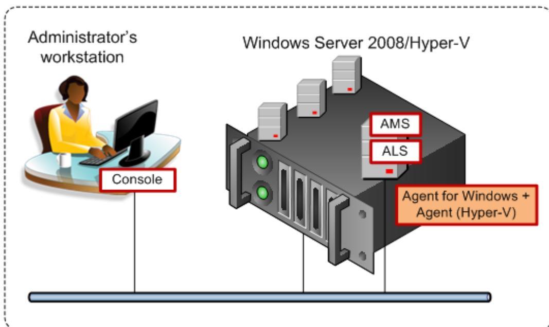
**AMS and ALS run on a regular virtual machine. Agent for Windows with the Agent for Hyper-V add-on runs in the host operating system. The administrator connects the console to the agent or to the AMS.**
