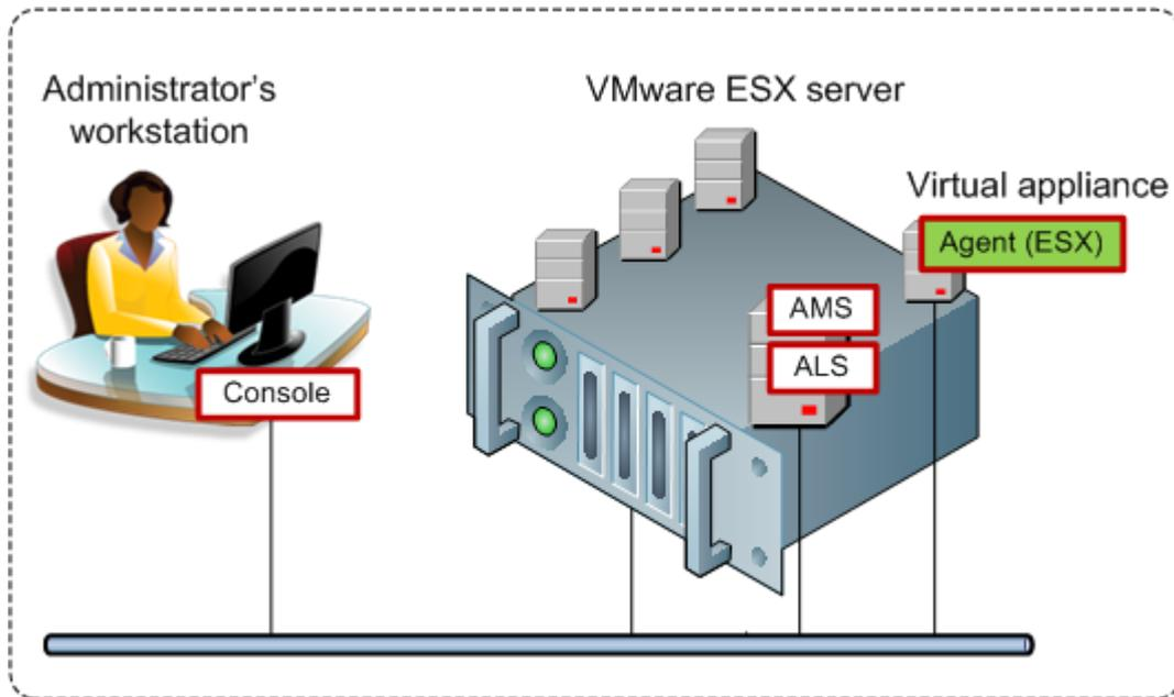
**AMS and ALS run on a regular virtual machine. Agent for ESX runs on a dedicated virtual machine called a virtual appliance. The administrator connects the console to the agent or to the AMS.**
